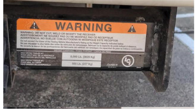
10.8 Item 2 (Picture) rear hitch capacity warning label
