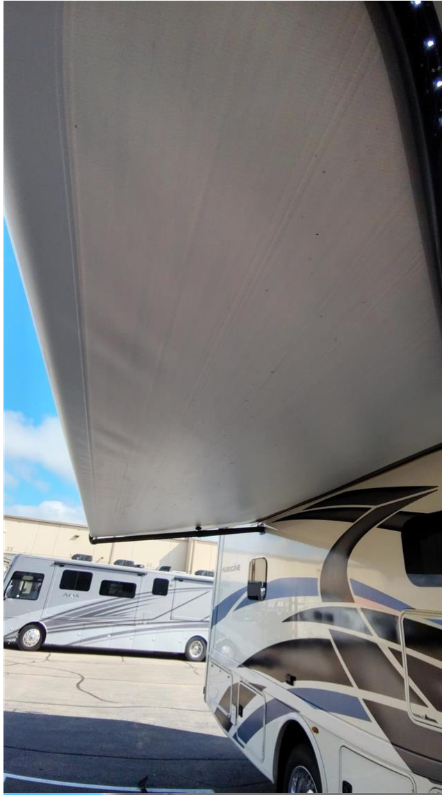
7.0.A Item 4 (Picture) Awning fabric condition underneath
