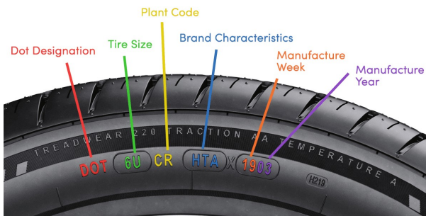
28.0.D Item 1 (Picture) Typical DOT Tire Codes Annotated
