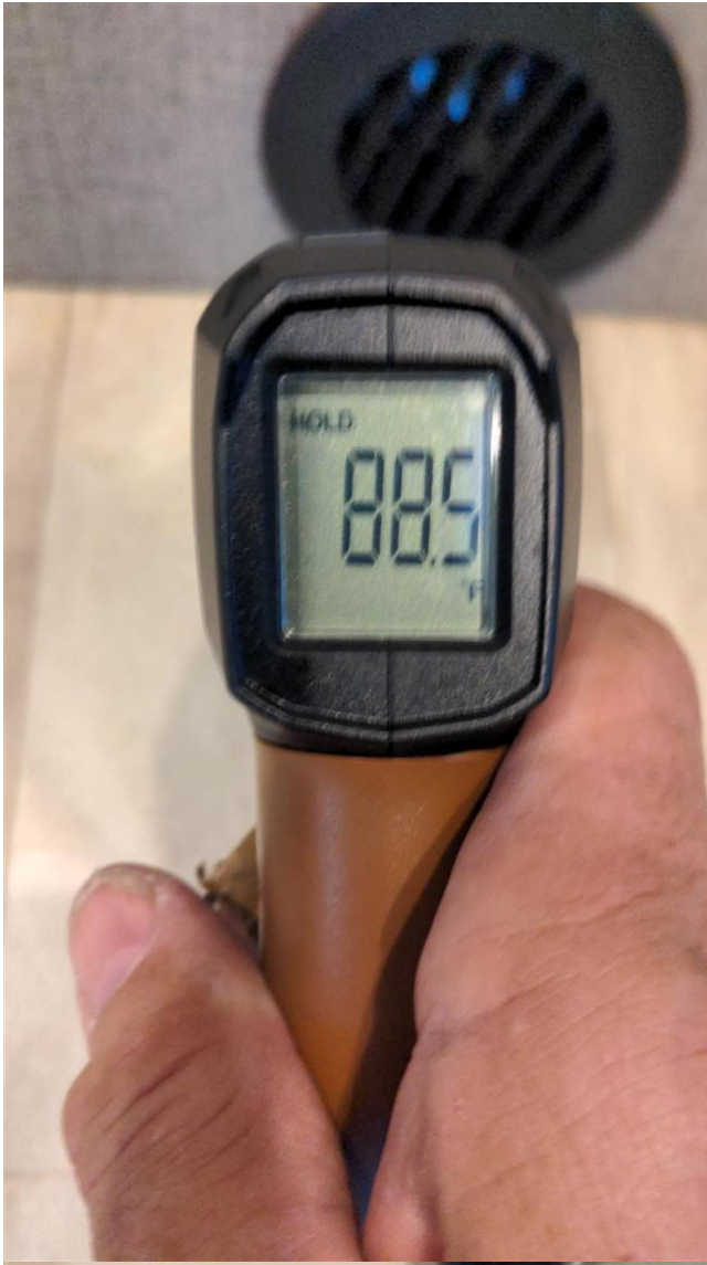
18.0 Item 1 (Picture) furnace air temperature
