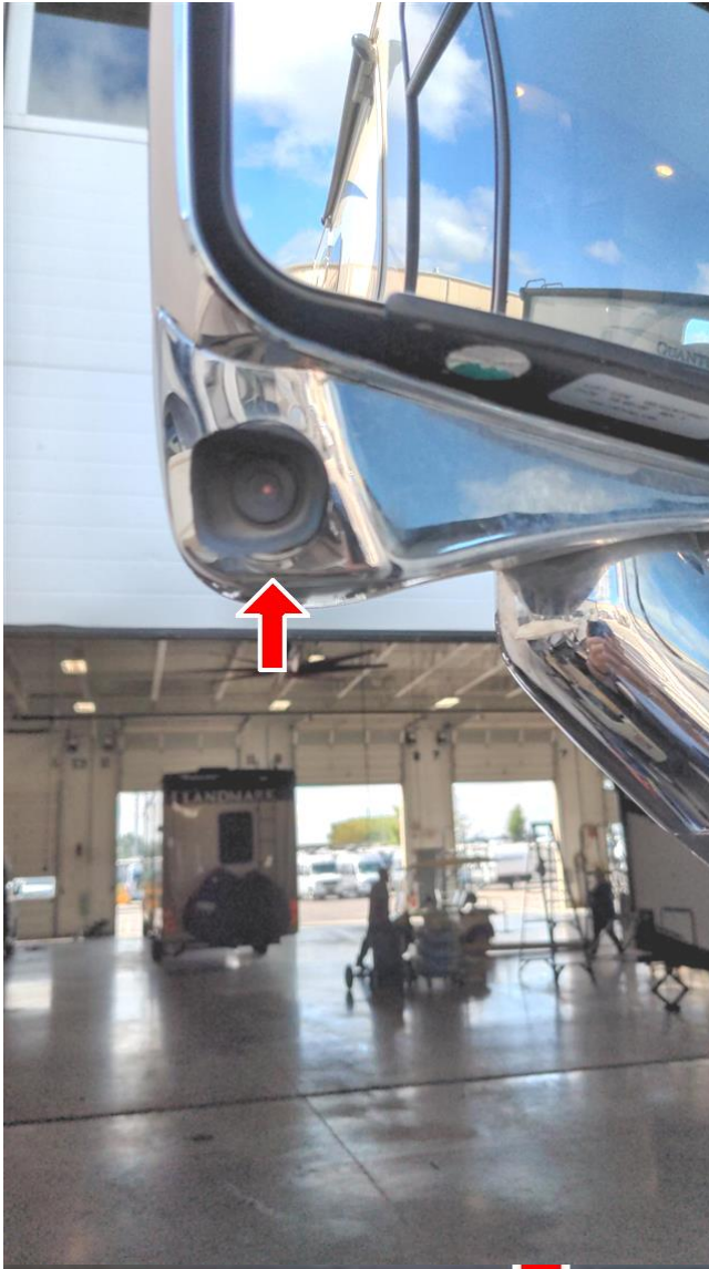
11.3 Item 1 (Picture) streetside sidewall camera
