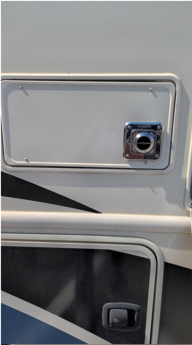
13.3 Item 1 (Picture) exterior furnace vent
