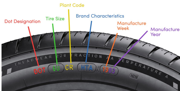
28.0.B Item 1 (Picture) Typical DOT Tire Codes Annotated
