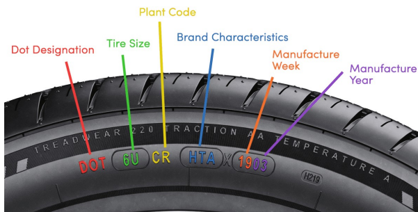
28.0.E Item 1 (Picture) Typical DOT Tire Codes Annotated
