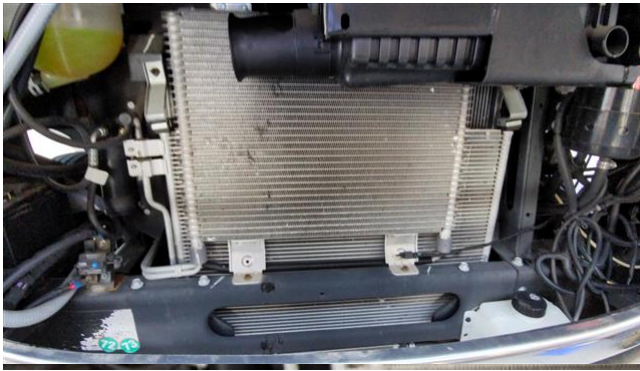
26.2 Item 1 (Picture) radiator
