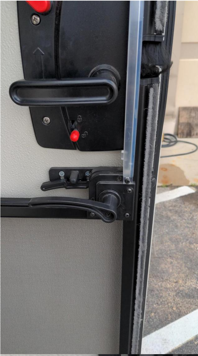
6.7 Item 4 (Picture) door handle lock unlocked
