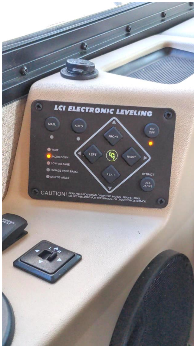
25.0 Item 1 (Picture) leveling Control pad
