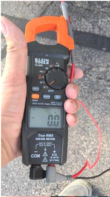
2.5 Item 1 (Picture) chassis voltage
