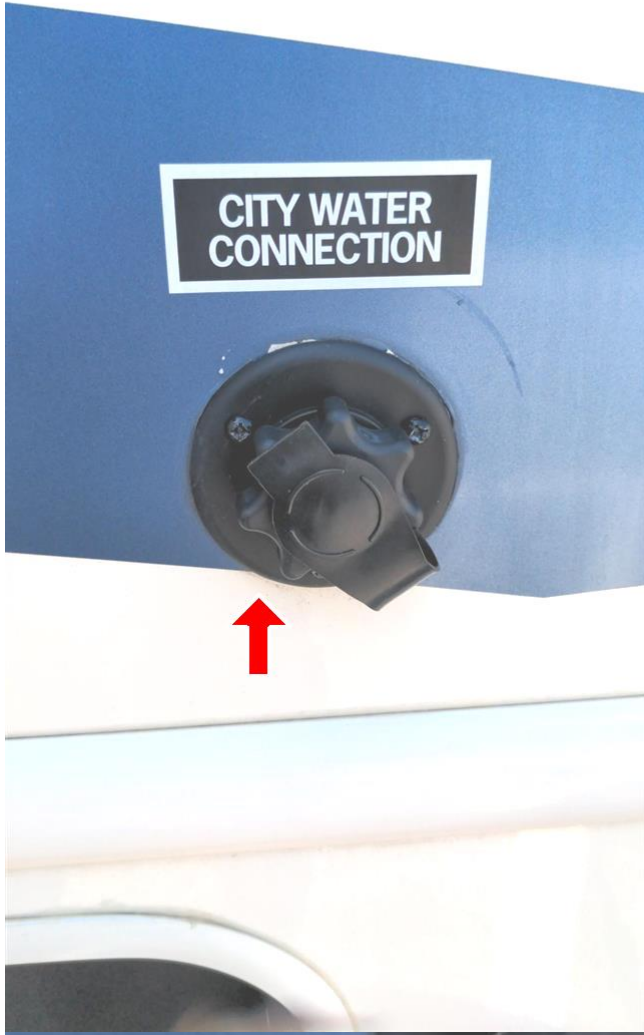
14.2 Item 1 (Picture) city water connectioncity water connection
