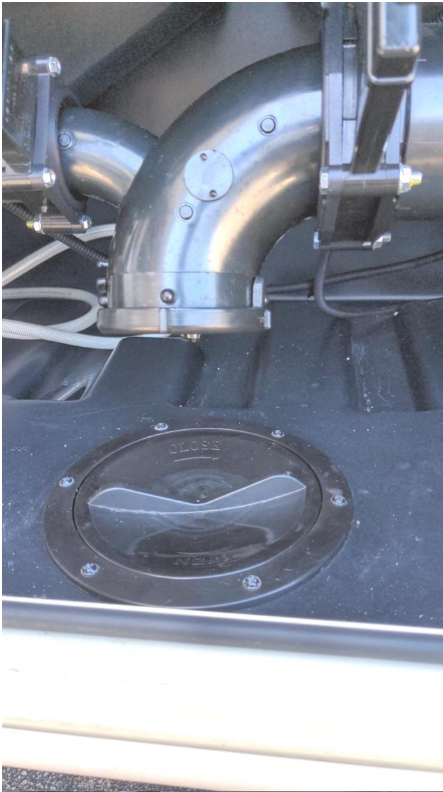
14.7 Item 1 (Picture) sewer hose fitting
