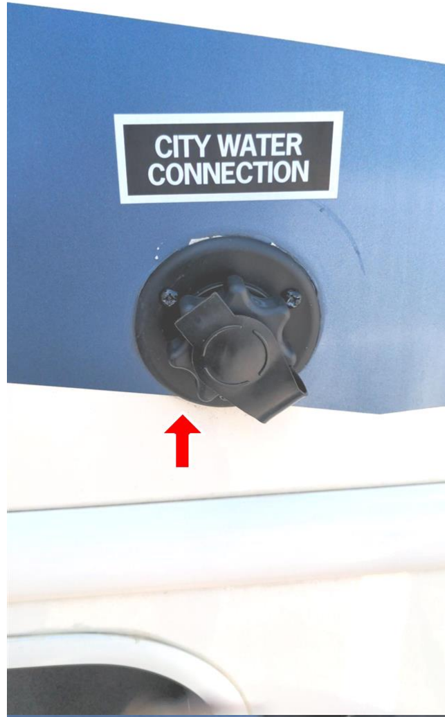
14.2 Item 1 (Picture) city water connectioncity water connection
